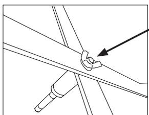
Secure stem with washer and screw at bottom of base
