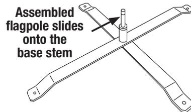
Assembled flagpole slides onto the base stem
